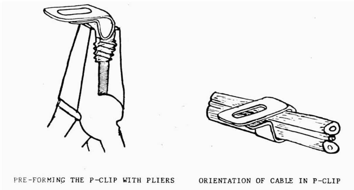
16) Place the P-Clip on the arm cable, about 6 3/4 inches from the plug, (Distance not critical.) Orient the cable in the P-clip so that its wide dimension will run vertically, per the illustration.
